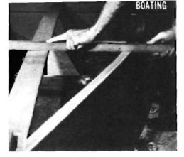
The final job before the bottom goes on is that of checking the planing job with a "fairing" stick, which measures flatness for installing the bottom.
