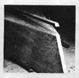
Outer keel goes on last, covers any gap between bottom halves, seals bottom, good launching skid.
