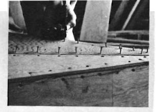
To strengthen hull, cover exposed bottom side joint with a strip of lumber for chaffing quard.
