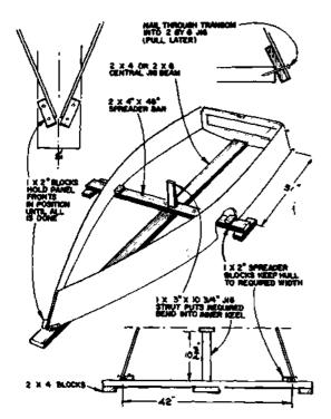
With inner keel secured to side panels, front end glued and screwed, chine rails are then bent in (as shown here), ready for securing to Interior sides; the 3/16-mch exposure is to be planed.
