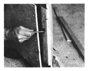
With the front bow aligned and drilled, glue and \*crew It closed, as described. Note that two chine rails with planed bevels are now ready to be wedged into place. Study the diagrams ior details.
