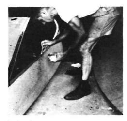
Weldwood mix is brushed on at this point. Note that half of bottom is already secured in place.
