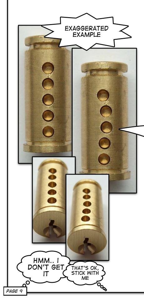
LOCK PICKING WORKS BECAUSE OF A VULNERABILITY CREATED BY MECHANICAL TOLERANCES IN THE MANUFACTURE OF LOCKS. SMALL MISALIGNMENTS IN THE PIN CHAMBERS, CHAMBERS THAT ARE MISSHAPEN (OVAL), AS WELL AS MISSHAPEN PINS WILL CREATE WHAT IS CALLED THE BINDING EFFECT (EXPLAINED NEXT).
