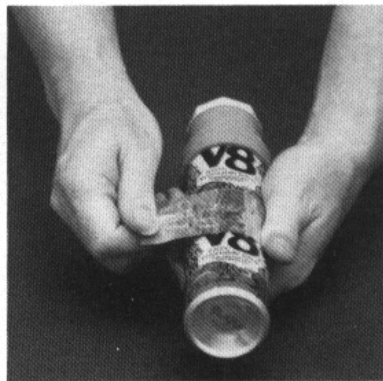
Tape second can onto first with metal repair tape.
