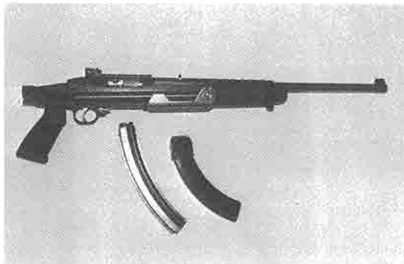
Right side view of the newly converted selective-fire Ruger 1022. This one sports a folding stock which is shown in the folded position. A 30-shot, banana-type clip and a 25-shot Eaton magazine are below. Selector is set at "full auto."
