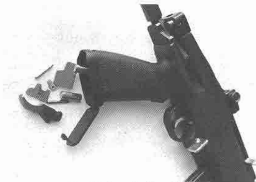
View of the folding stock pistol grip cover hinged open. This compartment can easily accommodate spare parts for the conversion or store the original trigger mechanism.
