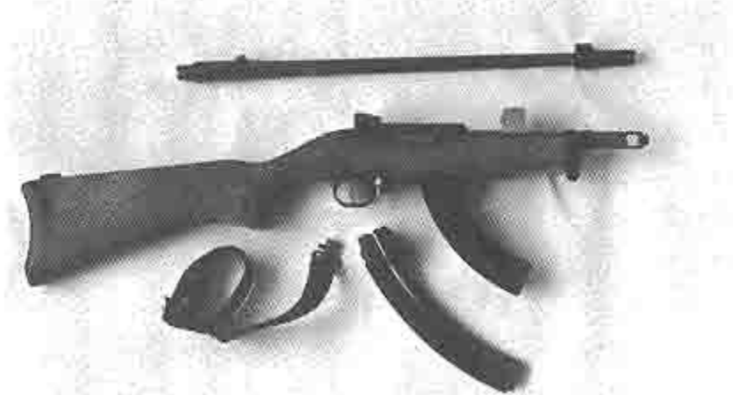
The ultimate 1022 weapon system. Photo showing the short SMG configuration with standard 18 1/2-inch barrel with flash hider, military sight system, 30- and 25-round clips (50-round drum magazines are now available) and side-mounted assault sling. The winner for the "affordable alternative" contest—a .22 rimfire full auto at its best!
