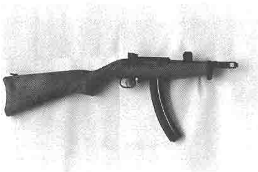
This ultra short SMG configuration of the selective-fire Ruger 1022 features the fully adjustable .30 caliber M1 carbine rear sight and a custom built UZI SMG-type front sight with protectors machined from solid block of steel. The muzzle brake is a copy of the latest Russian AK-74 assault rifle device.
