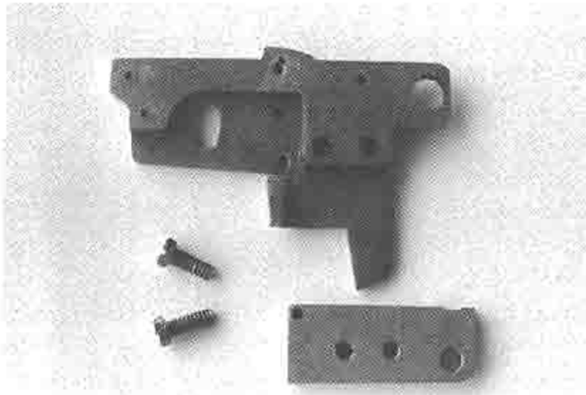
Close up showing a handmade three-piece sear. Parts are cut with a hacksaw then roughly shaped by files before being riveted. After fitting, parts are heat treated and polished.
