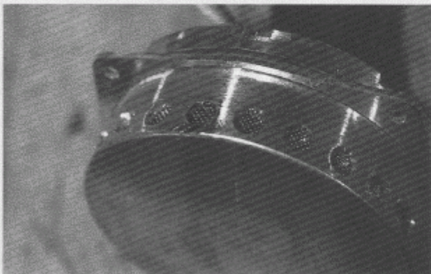
The aluminum detonating chamber is die-stamped together and cannot be disassembled nondestructively. The screened holes allow gas into the air bag.
