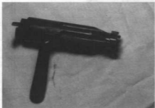
End view of the bolt. The locking lugs and ejector are visible (far right).
