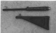
Interchangeable barrels and detachable buttstocks, making a rifle and pistol combination, can be desirable features. However, if the short barrel is in place when the buttstock is added, an illegal weapon will result.
