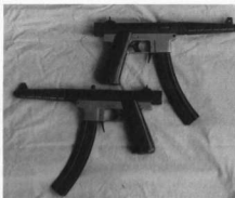
Commercial magazines made for use in the Thompson .22 were used in my MP22 pistols (above).
