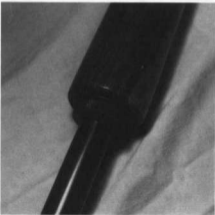
A knurled barrel nut threaded on the barrel holds the forend in place.
