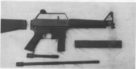
A 9mm conversion unit on an AR-15/M16 lower receiver shown with a detachable butt stock; 16-, 10- (mounted), and 6-inch barrels; and 15- and 30-round magazines. Using an original M16 receiver to make a 6-inch-barrel pistol is making a "short-barreled rifle" according to the BATF.
