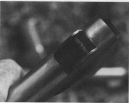
Rear sight made of folded sheet metal and silver soldered in place, as used on assault-type pistols.
