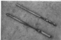
Long drills to bore stock holes.
