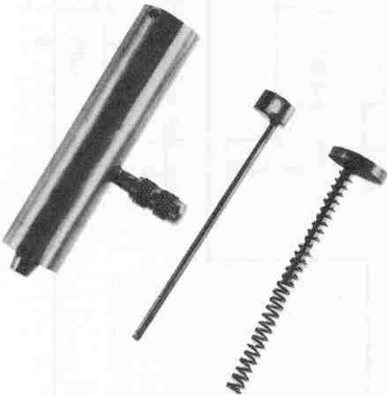
The bolt must have an offset recoil spring. Full-length firing pin.
