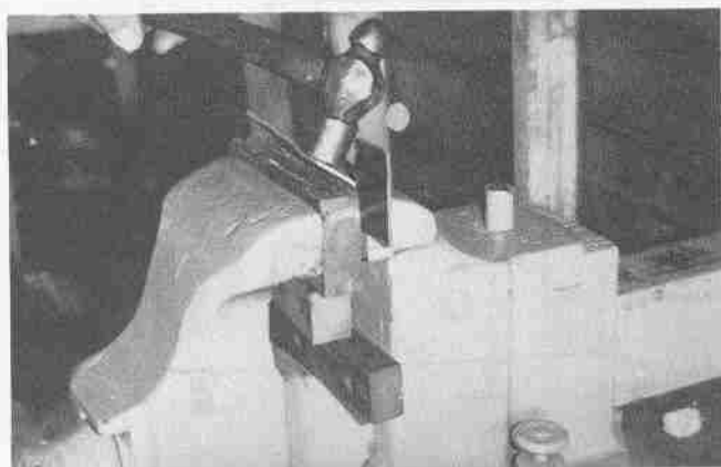
The flange, which will form the lower side, is folded 90 degrees with a heavy hammer.
