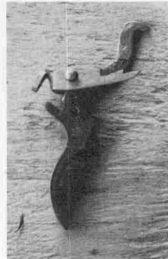
Trigger with trigger bar pinned in place.
