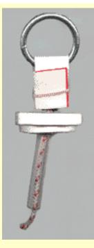
Slip a length of 1/2" O.D. or so plastic tubing cut to such length that a quarter inch of fuse end is exposed. Center the fuse in the tubing and pack the space between with small beads of wax that are hand softened and pressed in with a small stick. This is to prevent premature explosion from fuse blow by.
