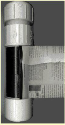
Next, a paper envelope is made from newspaper cut to such width that it can be folded in half with an extra 1/2" that folds back over the open edge, and still fit between the coupler and end cap. The paper envelope is about 1' in length.
